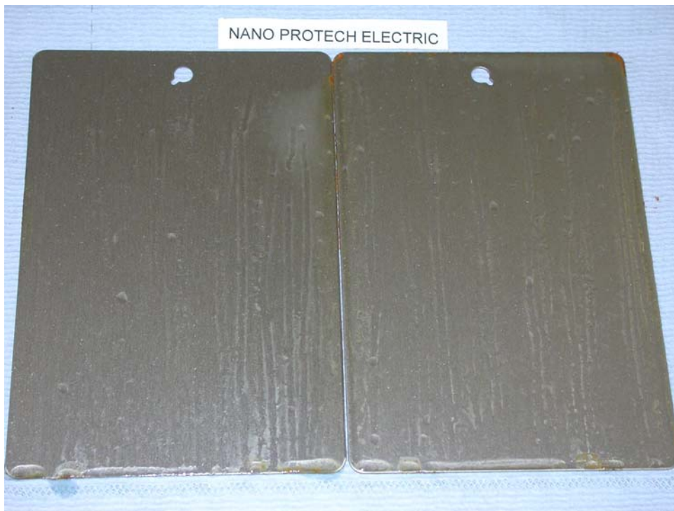
Photograph showing the condition of the Nano Protech Electric Test Panels after 72 hours Salt Spray Test
