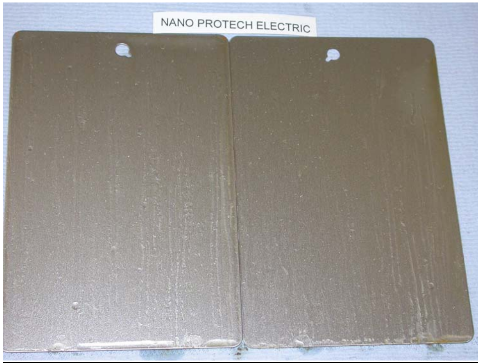
Photograph showing the condition of the Nano Protech Electric Test Panels after 48 hours Salt Spray Test
