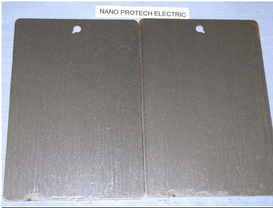
Photograph showing the condition of the Nano Protech Electric Test Panels after 96 hours Salt Spray Test
