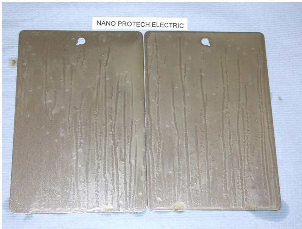
Photograph showing the condition of the Nano Protech Electric Test Panels after 24 hours Salt Spray Test
