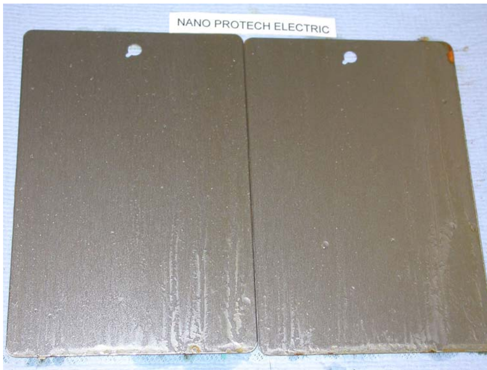
Photograph showing the condition of the Nano Protech Electric Test Panels after 48 hours Salt Spray Test
